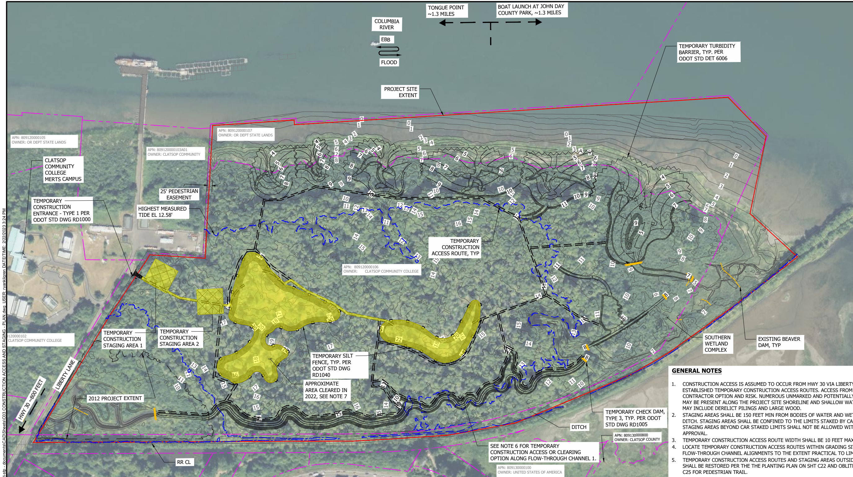
1 CONSTRUCTION ACCESS AND STAGING - PLAN Scale: 1:150
