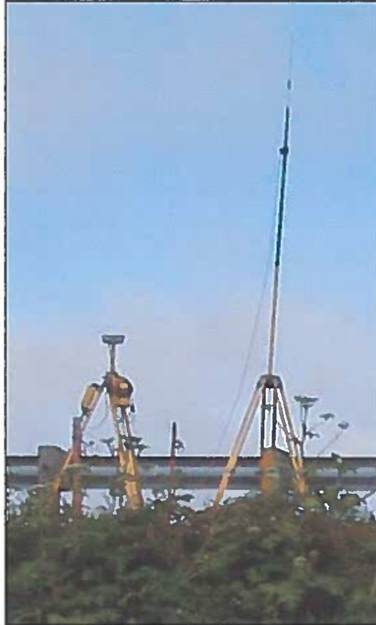
Figure 3-2. RTK - GPS base station deployed on the earth dike near Bear River
