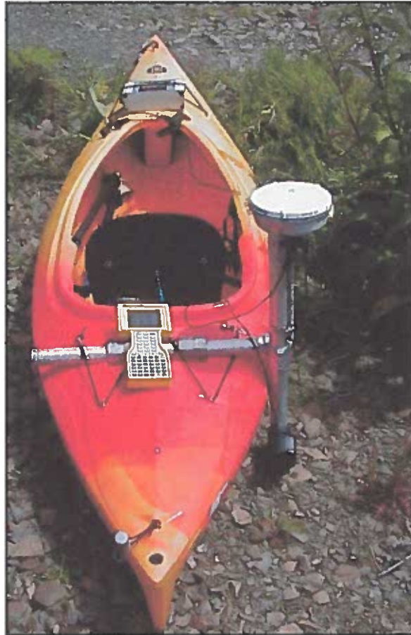
Figure 3-4. Kayak with GPS Rover unit and internally recording depth sounder
