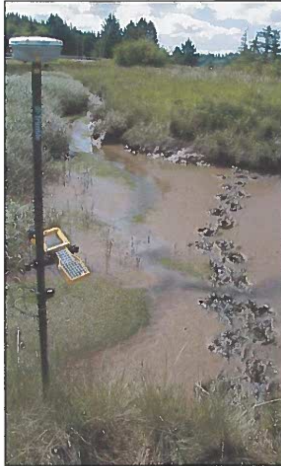
Figure 3-3. RTK-GPS survey rover station in use at Bear River project site
